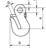
The first grade 100 eye shortening safety grab hook which prevents the accidental release of the chain whilst still providing no deration in capacity. This feature is useful when the chains have been loaded fully as there is no possibility of the chain becoming dislodged from the grab hook. Meaning once you have adjusted the legs there is no need to adjust them again.
